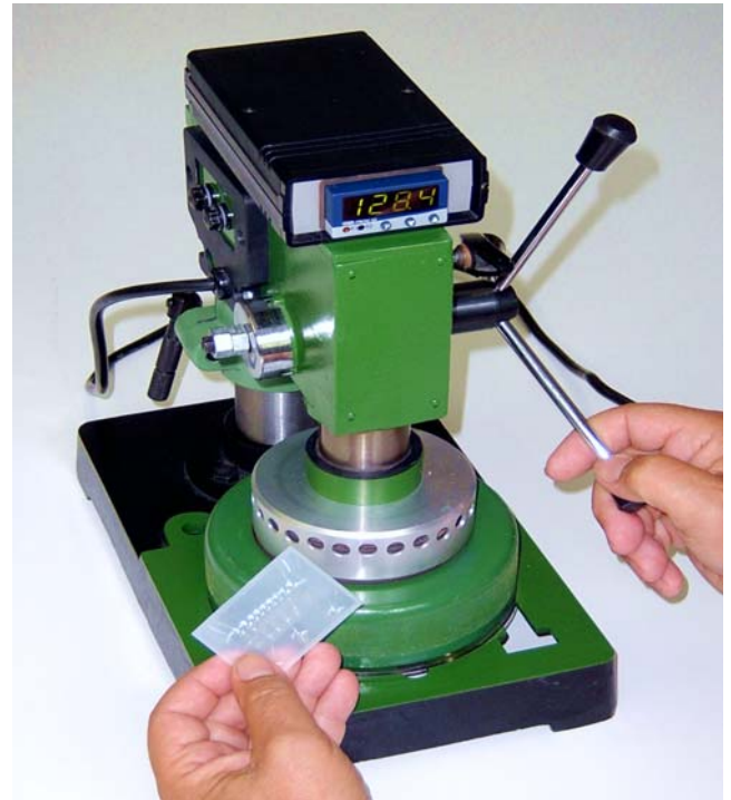
Hot press to make prototype fresnel lenses
