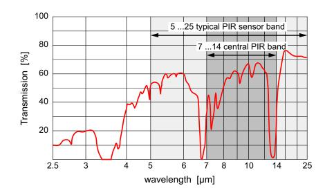
The low transmission at wavelengths below 3 µm helps to filter out unwanted daylight
