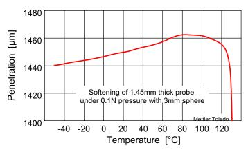
The TMA analysis shows the excellent dimensional stability of KUBE granulates over a wide temperature range
